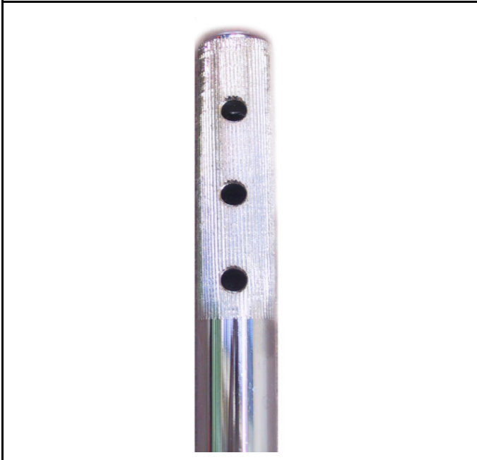
Above: photo of the steering column with the section with the knurling for the steering wheel hub (knurling according to DIN 82 - RAA1).
