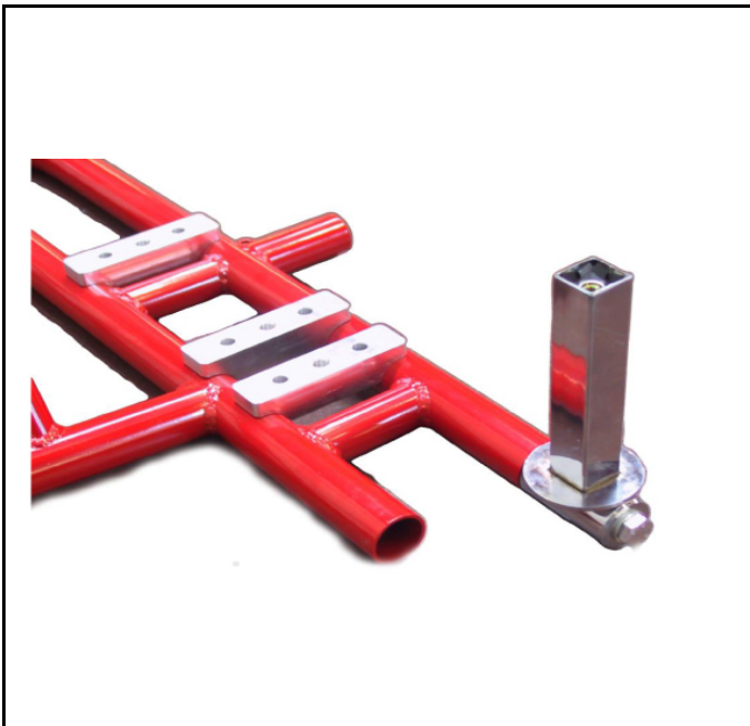
Above: photo of the frame from the side with the section of the support for the RTPS (Rear Tire Protection System)
