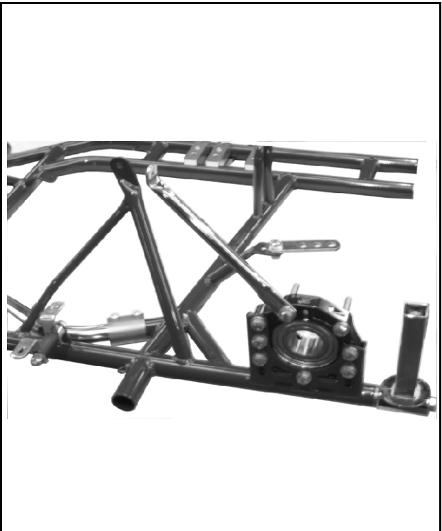
Foto of the frame from the side with the section of the supports for the radiator (radiator mounted) Radiator mounting position is 25^{\circ} \pm 5^{\circ} .
