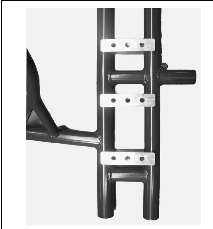
Foto from above of the frame with the section of the engine mount
