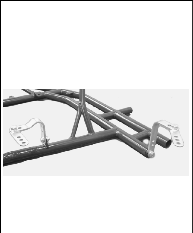
Photo from above of the frame with the section of the two supports for the exhaust system
