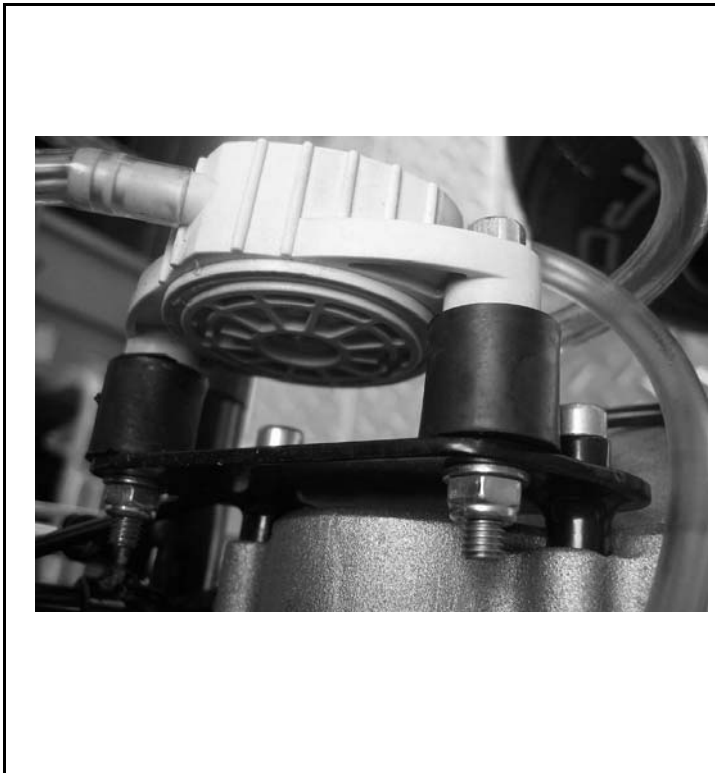
Photo of the frame with the section of the support for the fuel pump (fuel pump mounted)
