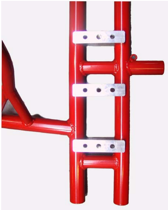
Foto from above of the frame with the section of the engine mount
